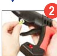
**2** Insert into the thermostat adjustment screw on the underside of the gun. Turning the screw fully anti-clockwise reduces the temperature to 130°C, while turning it fully clockwise increases it to 200°C
