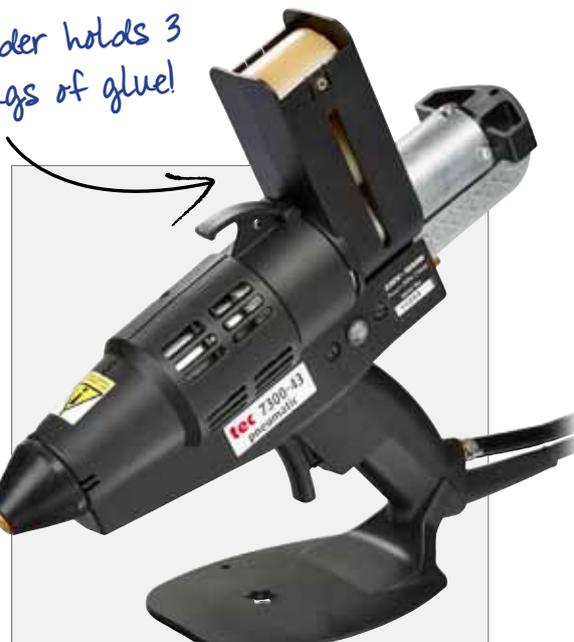
Extremely robust 43mm (1¾") spray glue gun with power-on light. Designed for industrial use, it sprays hotmelt at any angle with adjustable spray pattern. A non-toxic adhesive spray system, it covers large areas and applies hotmelt to heat sensitive substrates without damage. 7 bar (100psi) 85 l/min (3 cfm) air supply required.
