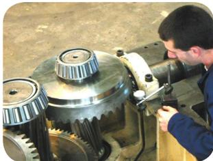
Permabond adhesives are ideal for bonding gears to shafts, repairing and replacing spun bearings, bonding bushings and sealing and gasketing gear box housings.
