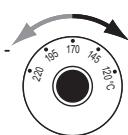
Use the included screwdriver (9) to set the temperature at the turning knob (3) to the desired value.
