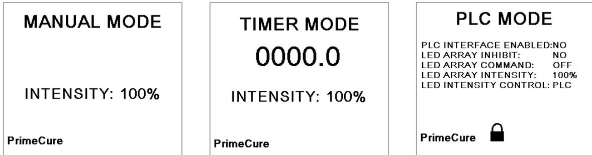
**NOTE:** If the BlueWave LED Flood System powers up in PLC Mode, you cannot change any settings via the front panel controls until you press the PLC Access Switch on the back panel.
