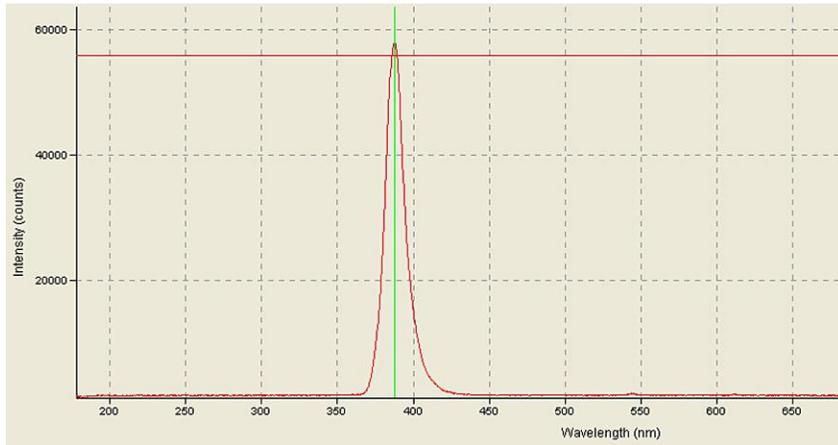
**Figure 31. BlueWave LED Flood with VisiCure® Array – 405 nm Spectral Output**
