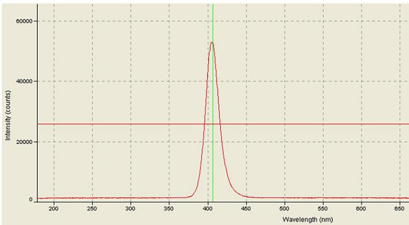
**Figure 32. BlueWave LED Flood with RediCure™ Array – 365 nm Spectral Output**
