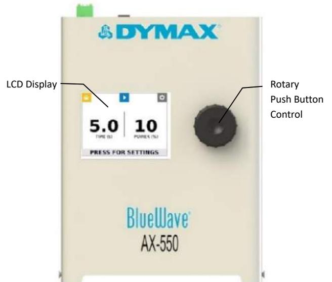
**Note:** The selected value will appear in blue color, when selected value requires modification press the rotary pushbutton, then, this value will turn yellow indicating it is ready to be modified. Turning the rotary pushbutton changes the value to be selected.
