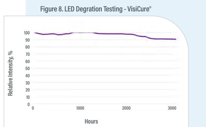
Note: Testing conducted at 70°F +/-3°F and 30% +/-10% Relative Humidity
