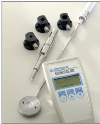
**ACCU-CAL™ 50 Radiometer**
