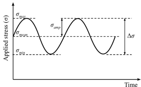
Figure 1: Cyclic loading of fatigue testing (Bastidas-Artega)
