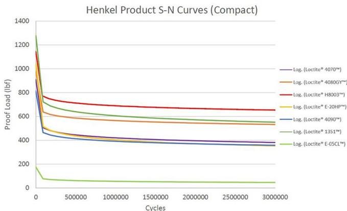
Figure 3: S-N Curves of Henkel Products Below 3 Million Cycles
